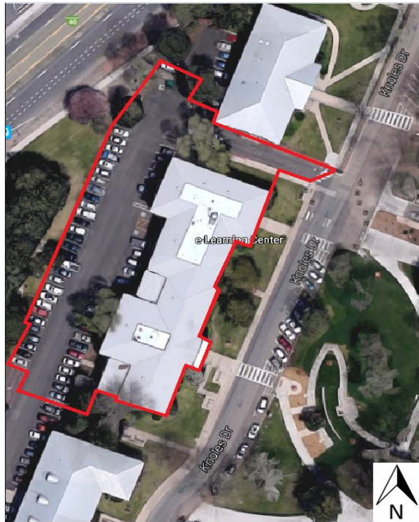
Figure 2: Basin Delineation for Gammage Building
